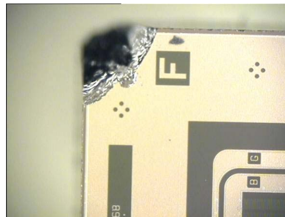
Corner chip damage
