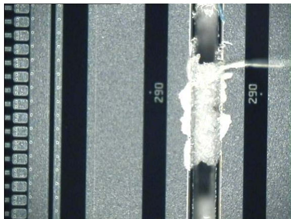
Minimal glue leakage
